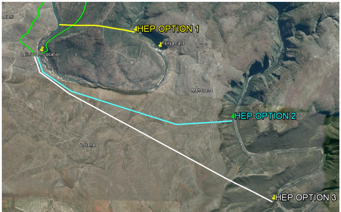
Figure 8: Hydropower Water Transfer Conduit Options
